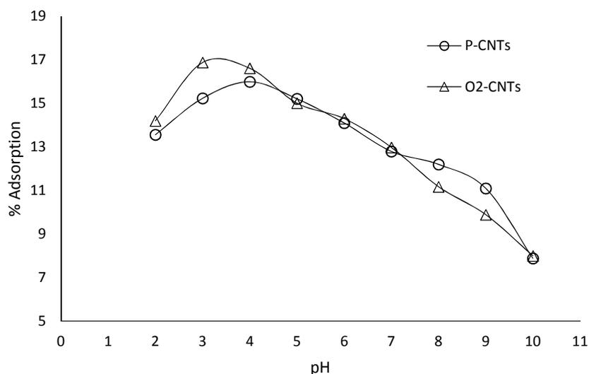
Fig. 1. Effect of pH on adsorption of MO on P-CNTs and O2-CNTs, time= 40 min,  $C_o= 10$  mg/L
