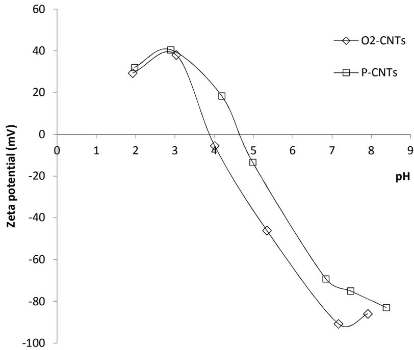
Fig. 3. Variation of zeta potential for O2-CNTs and P-CNTs as a function of pH and determination of pzc
