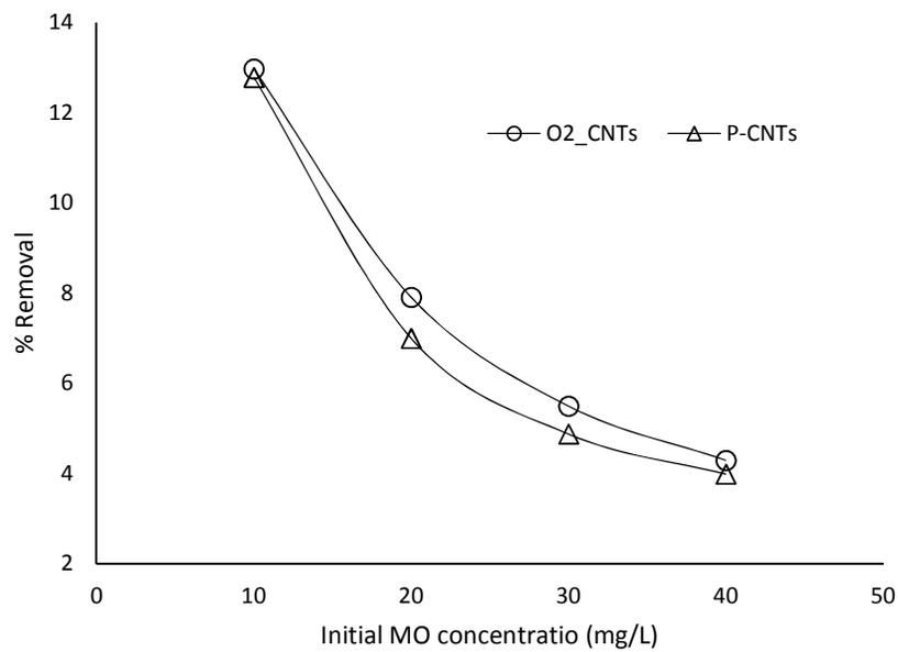
Fig. 4. The effect of initial concentration of MO on removal percentage at time = 40 min
