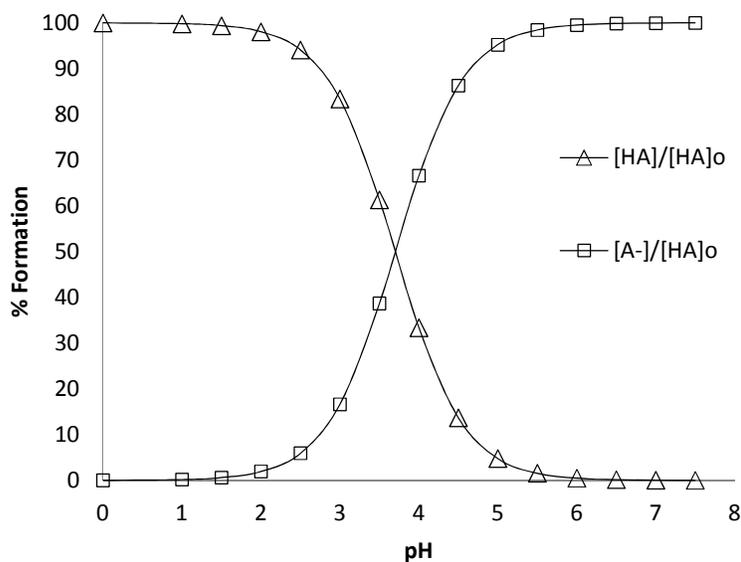
Fig. 2. The speciation curve of methyl orange
