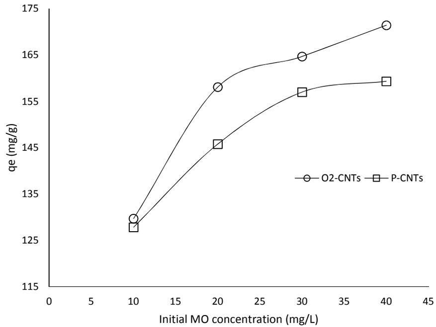
**Fig. 5. The effect of initial concentration of MO on  $q_e$  at time = 40 min**
